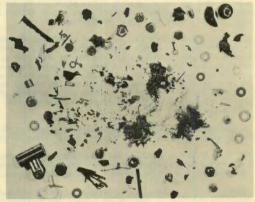
tanks mysteriously fell off during an in-flight refueling. A piece of this junk apparently bounced onto the terminal strip while the pilot was trying to mate probe and drogue and energized the jettison circuit.
